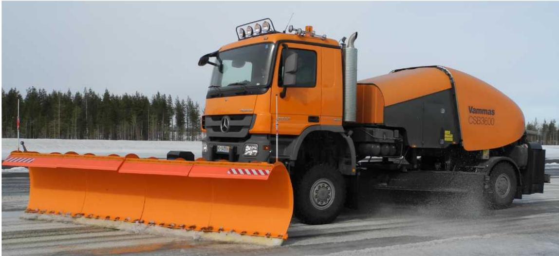
The VAMMAS CSB 3600 Compact Sweeper Blower has been designed for runways, taxiways and aprons. The CSB 3600 has been built on modified MERCEDES - BENZ ACTROS 2032 A 4x4 chassis. This allows the operator to have the best possible visibility. The 5.6m plow has a segmented design with poly or steel cutting edges. The 4.2m sweeper broom has been placed between the axles of the vehicle. The air blast for has been placed behind the rear axle to ensure all debris is removed.
