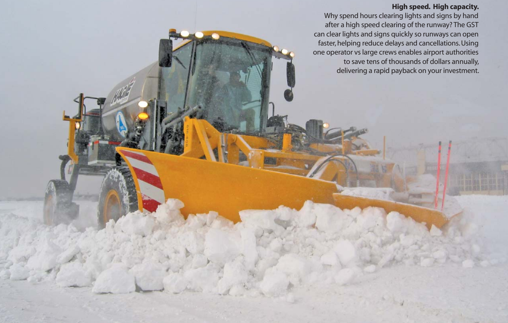
(A) As the operator approaches an edge light or sign, the plow pivots open, allowing two hydraulically-powered brushes to clear snow and ice with ease.
